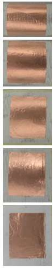
Fig. 5. Rectangular length-bent resonator 36x27 mm on sample S2 with bent diameters s ∞, 65, 50, 50, 30 and 20 mm
